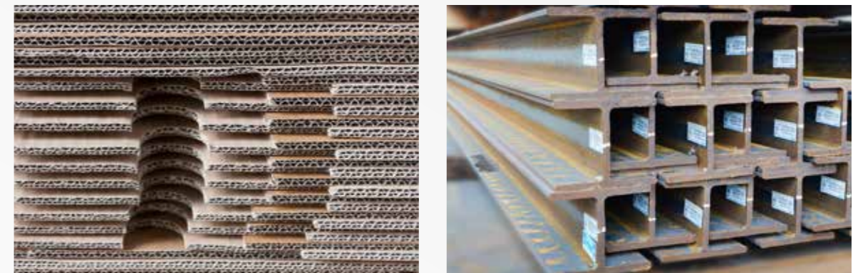
Practical examples of weight reduction at equal rigidity.
