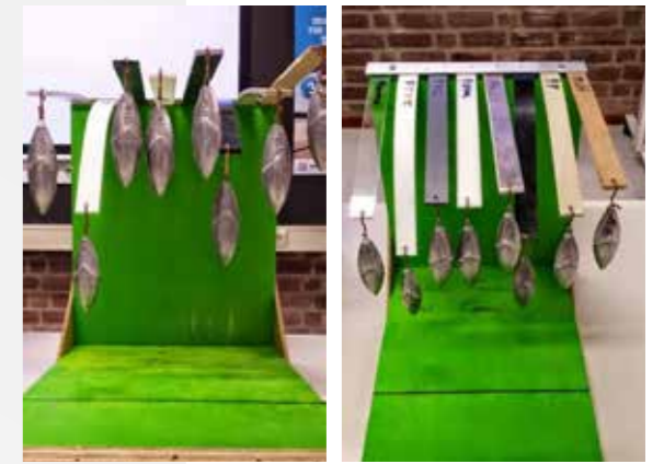
Experimental setup demonstrating creep.
